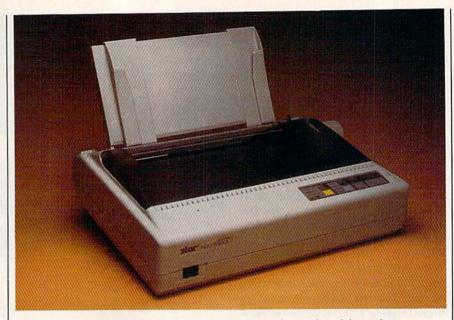
The Star Micronics NX-1000C Multi Font includes four onboard fonts that are selected from the front control panel.
